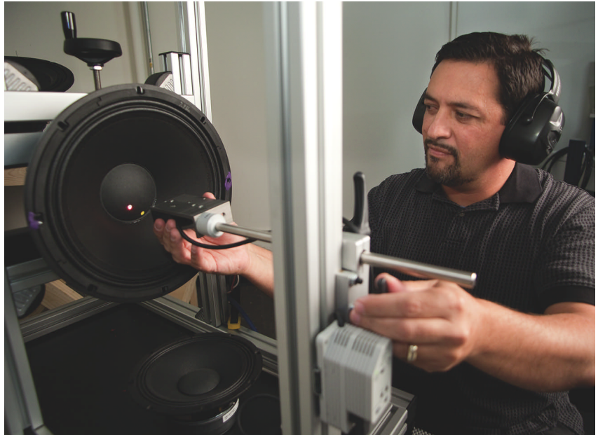
Luis Esparza tests transducers for loudspeakers by analyzing audio response and by measuring movement with a laser vibrometer.
