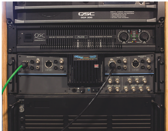
QSC's production test stations use audio analyzers from Audio Precision that make over 100 measurements.
